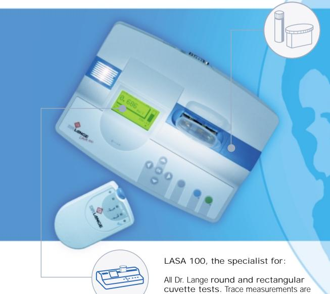
All Dr. Lange round and rectangular cuvette tests. Trace measurements are also child's play. In addition, LASA 100 makes special applications possible, such as turbidity and colour number measurements.
